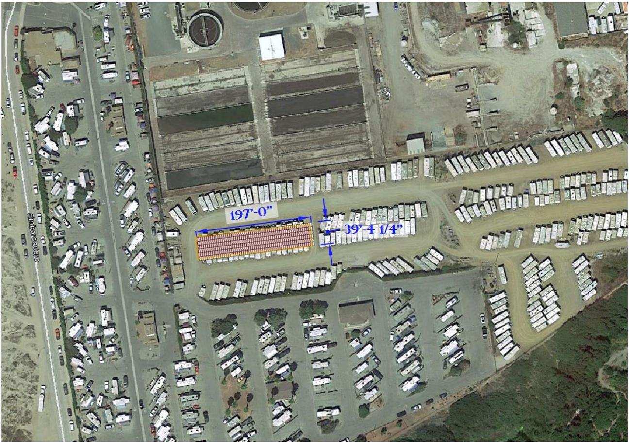
**SUBJECT REQUEST:** The lessee is requesting approval to install a solar carport over a section of parked trailers/RV's that are in storage. The carport facility will be approximately 37 feet wide and 197 feet long with a sloped shed roof that has a maximum height of 22 feet. The height allowed in the zone is 30 feet. The proposed facility complies with the development setbacks and height requirements for the zone.
