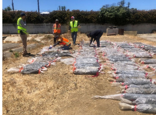
Well Site Cores (Deep Sonic Cores)
